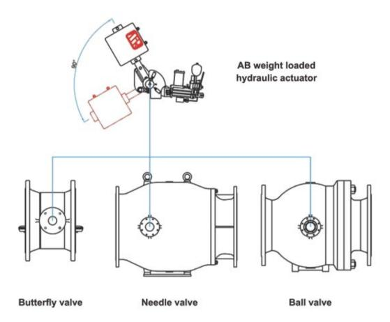
The weight loaded provides the energy required for a single closing or opening operating of the valve. **AB** compact type weight loaded Hydraulic Actuator is used for operating valves with a drive shaft rotating by max. 90 ,maybe incorporated in ball valves, Butterfly valves or needle valves. Range of size and standard interfaces combined with a perfect modular concept enable to supply the best solution for valves of all sizes and pressure ratings.
