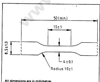
Figure 4. Dimensions of alternative dumb-bell
