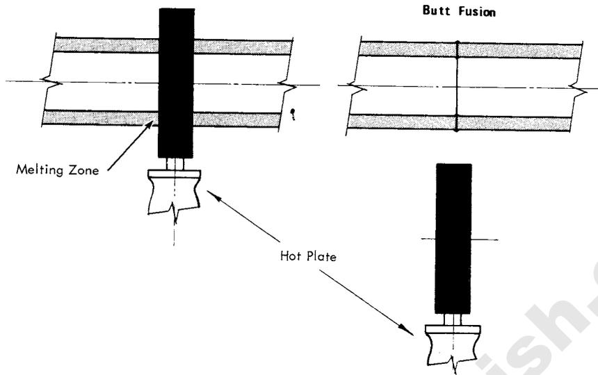
FIG. 2 Typical Butt Fusion Operation
