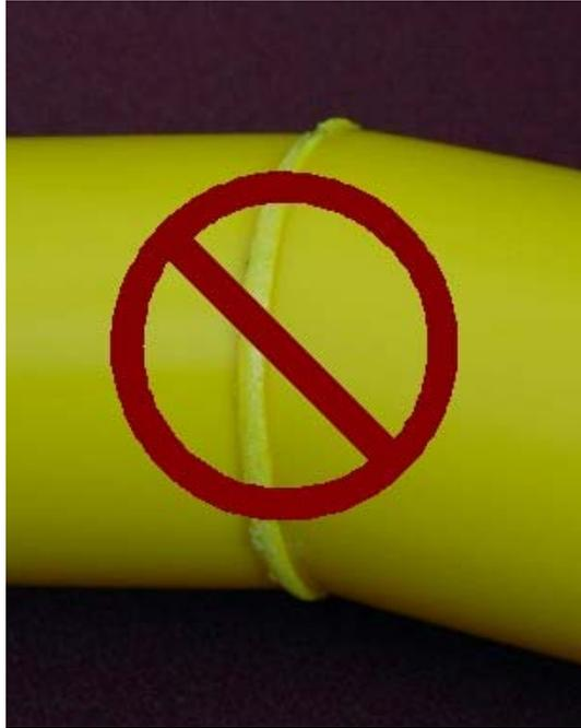
Figure A2 Visually unacceptable mitered joint
