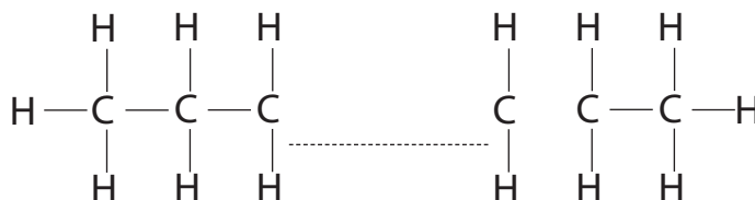
Figure 1-1c: Polyethylene Molecular Chain
