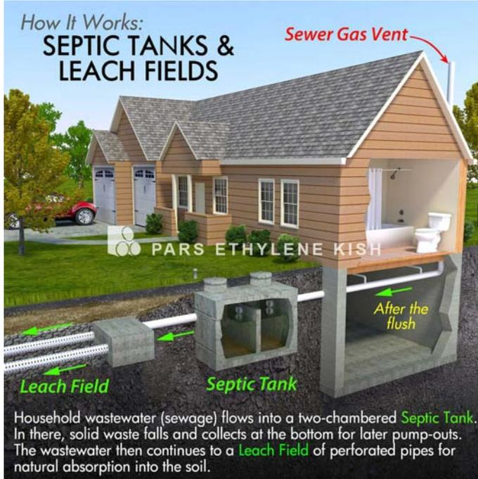
Household wastewater (sewage) flows into a two-chambered **Septic Tank**. In there, solid waste falls and collects at the bottom for later pump-outs. The wastewater then continues to a **Leach Field** of perforated pipes for natural absorption into the soil.
